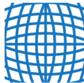
Positive radial distortion "barrel"
